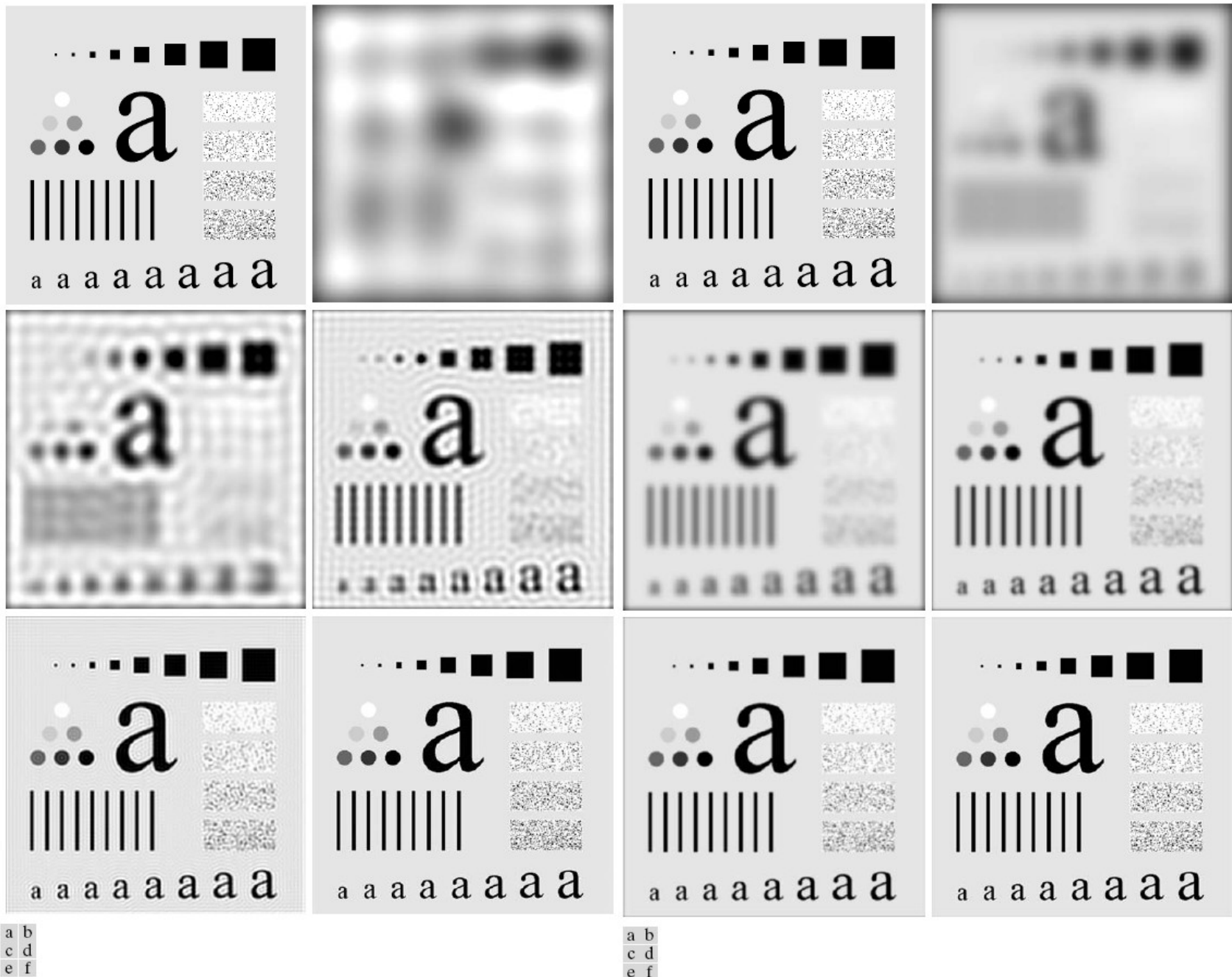
FIGURE 4.42 (a) Original image. (b)–(f) Results of filtering using ILPFs with cutoff frequencies set at radii values 10, 30, 60, 160, and 460, as shown in Fig. 4.41(b). The power removed by these filters was 13, 6.9, 4.3, 2.2, and 0.8% of the total, respectively.
