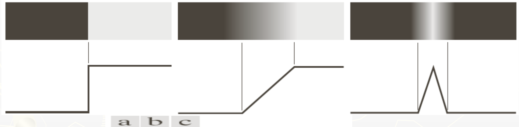
FIGURE 10.8 From left to right, models (ideal representations) of a step, a ramp, and a roof edge, and their corresponding intensity profiles.
