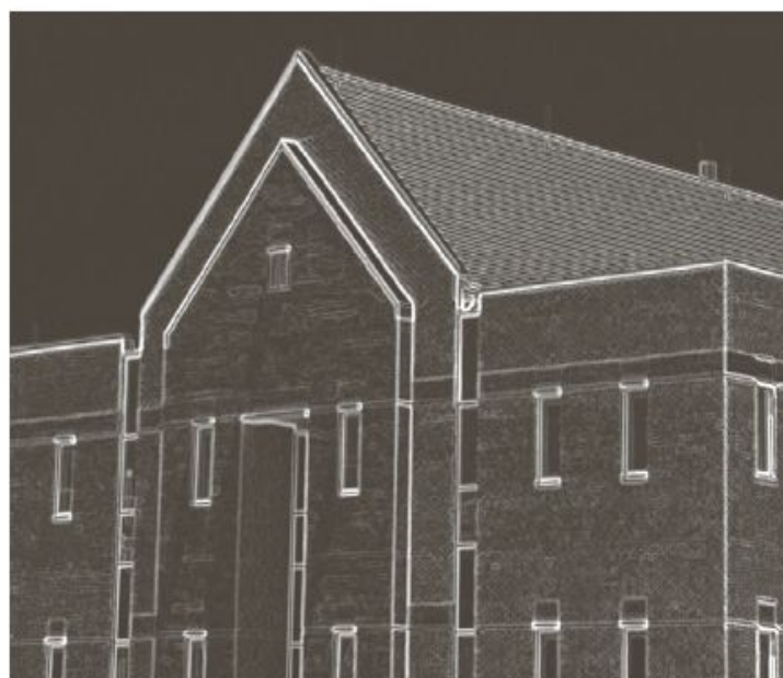
FIGURE 10.18 Same sequence as in Fig. 10.16, but with the original image smoothed using a 5 \times 5 averaging filter prior to edge detection.
