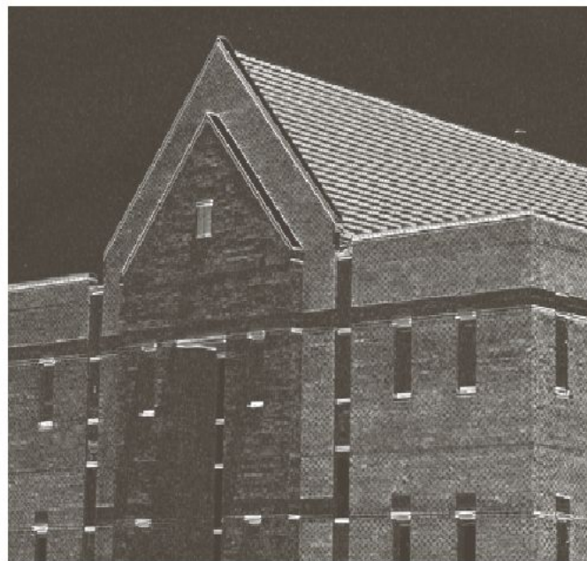
FIGURE 10.16 (a) Original image of size 834 \times 1114 pixels, with intensity values scaled to the range [0, 1] . (b) |g_x| , the component of the gradient in the x -direction, obtained using the Sobel mask in Fig. 10.14(f) to filter the image. (c) |g_y| , obtained using the mask in Fig. 10.14(g). (d) The gradient image, |g_x| + |g_y| .
