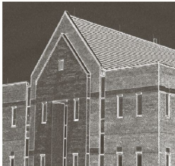
FIGURE 10.16 (a) Original image of size 834 \times 1114 pixels, with intensity values scaled to the range [0, 1] . (b) |g_x| , the component of the gradient in the x -direction, obtained using the Sobel mask in Fig. 10.14(f) to filter the image. (c) |g_y| , obtained using the mask in Fig. 10.14(g). (d) The gradient image, |g_x| + |g_y| .
